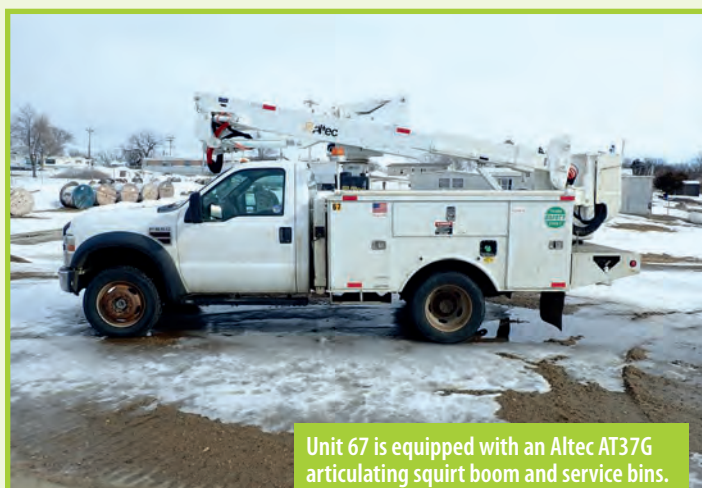
Unit 67 is a 2008 Ford F550 with 118,629 miles and an Altec AT37G articulating squirt boom. The engine is out.
